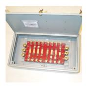
Fuse Panel, Navy Symbol 613, totally enclosed, 125 volts, three phase line, single phase loads, 8 circuit, no switches. Designed for maximum feeder of 75 MCM, maximum branch cable size 14 MCM. Enclosure is steel. Can be made in aluminum, if desired. Specify Symbol 613.1. Also can be modified for 480 volt applications.
