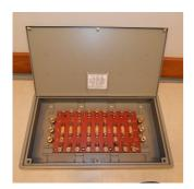
Fuse panel, Totally Enclosed, Steel, 450 Volts, 3 phase feed, 6 three phase branch circuits, for Type F15 (250 volt) or F61 (450 volt) fuses. Max feeder size 75 MCM. Max branch cable size 40 MCM. Symbol 545 per Mil-DTL-24646/4. Military Part Number M24646/4-003. NSN 5920-00-178-1626.
